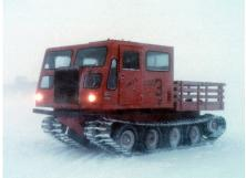
So how do they turn? These vehicles have two tracks, one on each side. There are motors attached to each track. If we make one track go faster than the other, then the vehicle will turn.
